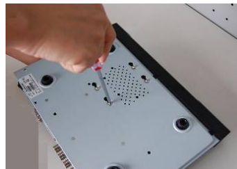
6. Fix the HDD firmly.
