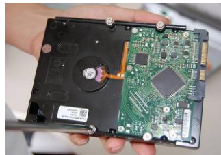
3. Rotate four screws three times to secure HDD bracket..
