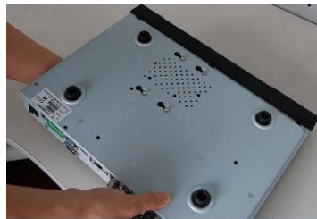
5. Turn the device upside down and then turn the screw in firmly.
