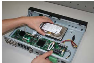
4. Place the HDD in accordance with the four holes in the chassis.
