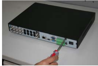
1. Loosen the screws of the upper cover.
