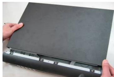
8. Close the upper cover and turn in the screws.
