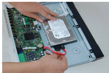
7. Connect the HDD cable and power cable.
